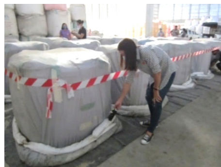
D) The phosphine concentration was checked daily using the Silo Chek
