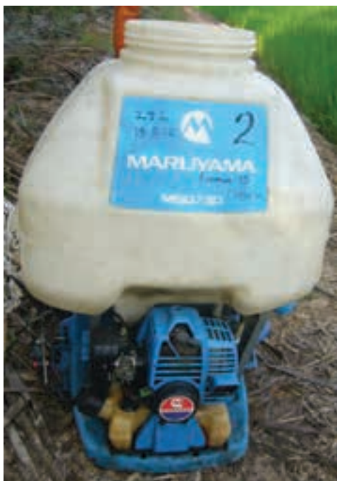
Figure 1 The sprayer used in the tests (a motorized hydraulic knapsack sprayer)
