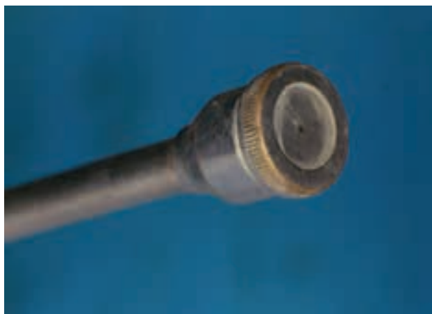
Figure 2 The nozzle used in the tests (a cone type nozzles, orifice sized 1.5 mm in diameters )
